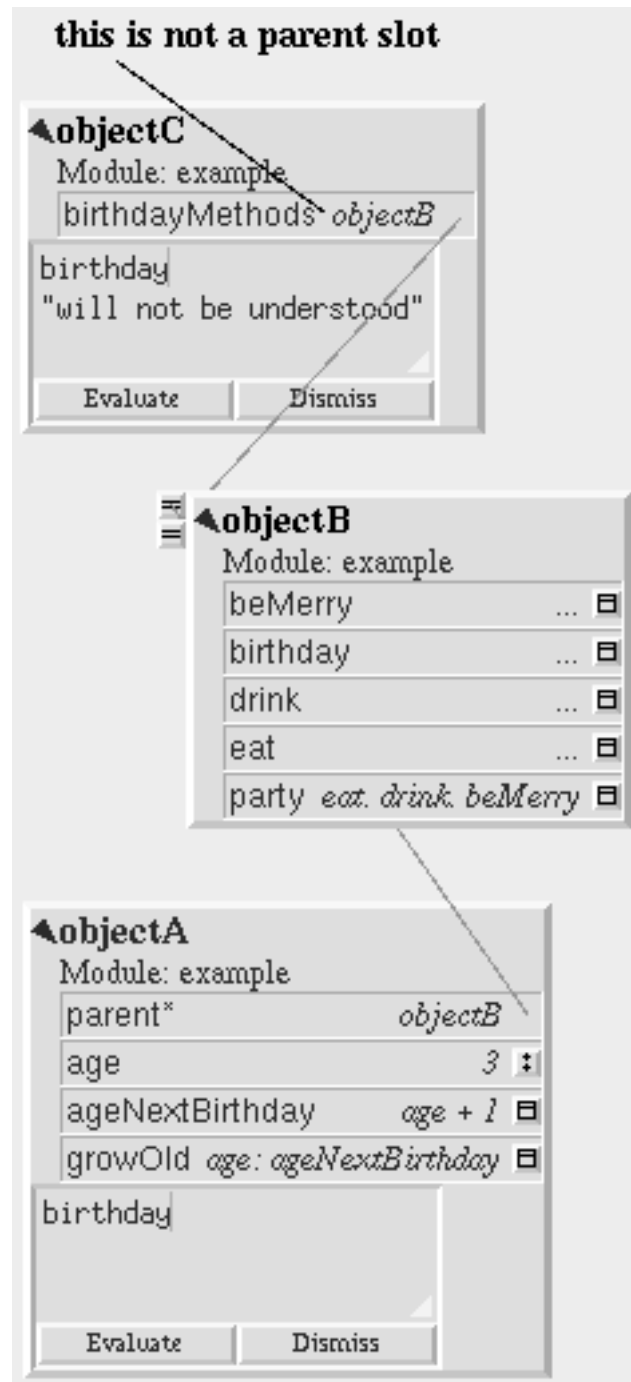
Figure 2.4: A parent object referred to by both a parent and non-parent slot.
